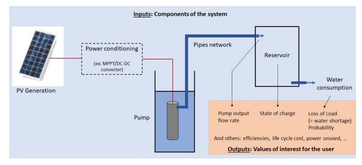
*Pvpumpingsystem* also offers to automate the process of sizing. In this case, the user can provide a set of PV module, a set of motor-pumps and a water needs file, and the software looks for the cheapest assembly while making sure that it respects a minimum risk of water shortage.
