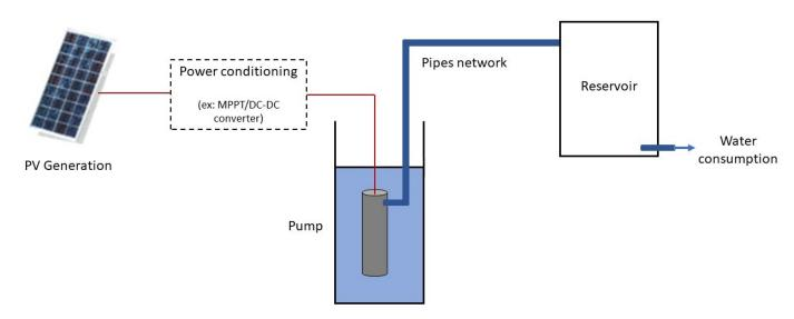
The simulation eventually compute numerous outputs like hourly flow rates of a given pump, efficiencies of components, risk of water shortage and life cycle cost of the whole system.
