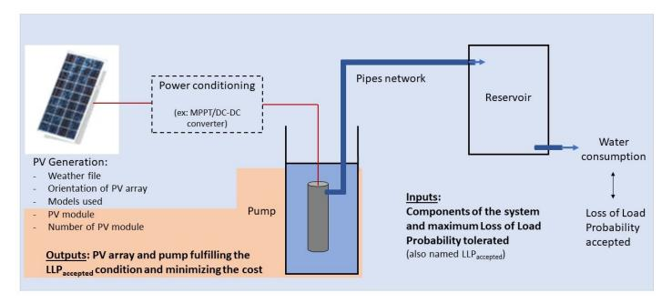
Nevertheless, the number of sizing processes can be infinite, and this module is expected to significantly expand with time, welcoming new sizing process based on different selection criteria or algorithms. In particular, the reservoir size, the orientation of the PV array, the coupling strategy or even the diameter of pipes are inputs that could ultimately become outputs of the sizing process as well.
